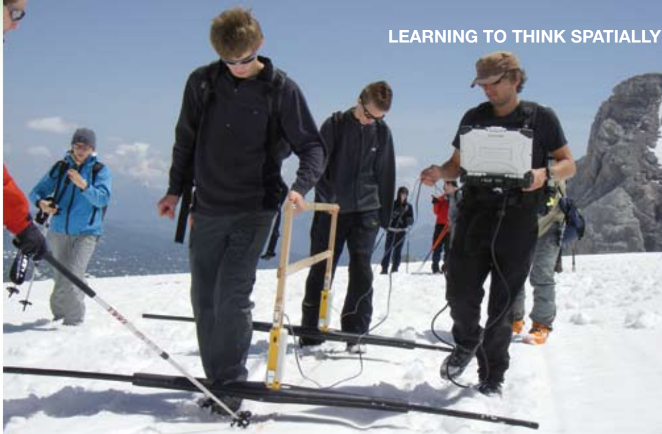
Pupils of BG Nonntal conduct measurements on Dachstein Glacier using Georadar, June 2008
