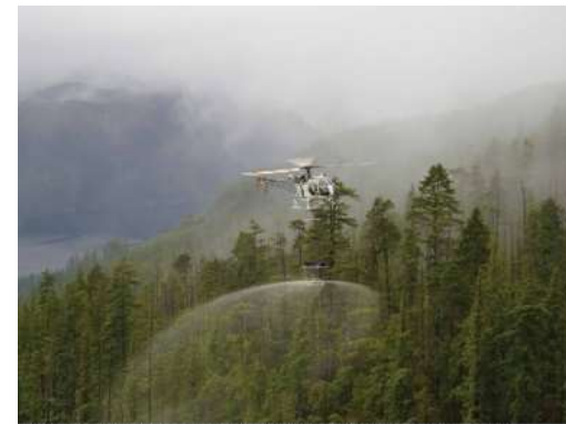
Western Aerial Applications utilizes three heavy lift Adrospatiale SA315B Lamas to fertilize replanted forests in mountainous regions of British Columbia. Western Aerial Applications Photo
